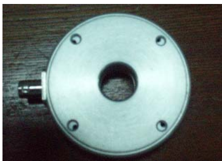
Fig. 9. The designed current transducer
