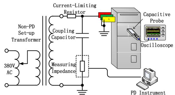
Fig.1. Testing circuit of PD
