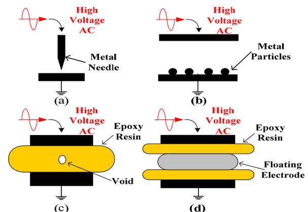
Fig.2. Artificial defect model
