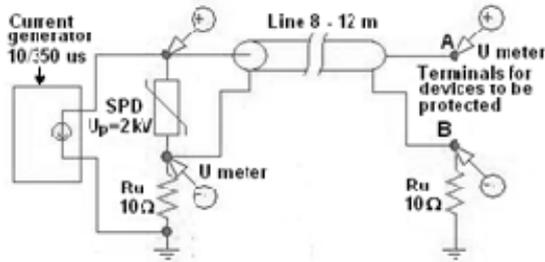
Fig. 3. Scheme of shielded arrangement with spark-gap used for PSpice simulations
