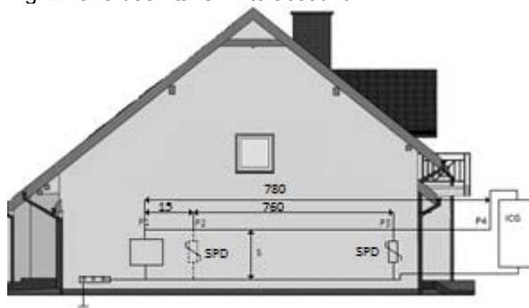
Fig. 1. Investigated arrangement (dim. are given in cm)
