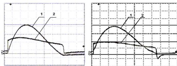
Fig. 6. Curves of voltages: a)  $U_{P1}$ , b)  $U_{P3}$ , registered in arrangement item 1) at beginning and  $U_1 = 3$  kV
