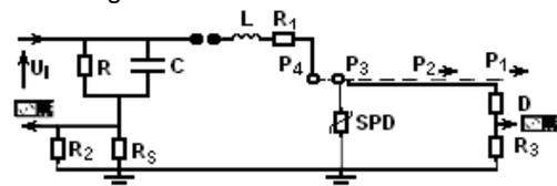
Fig. 5. Scheme of impulse current generator with measuring sets
