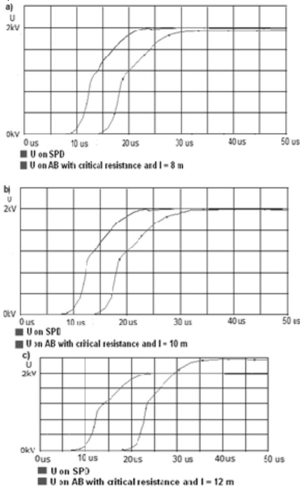
Fig. 4. An example of simulation: residual voltage on varistor for three different length of the wires between SPD and protected device ( $R = 10 \Omega$ ): 6a) 8m, 6b) 10m and 6c) 12m.
