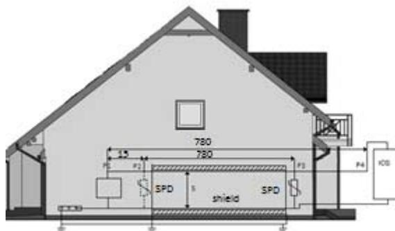
Fig. 2. Scheme of investigated shielded arrangement
