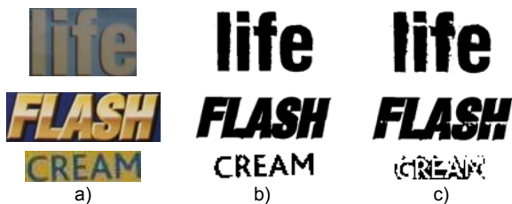
Fig. 5 Examples in which Euclidean distance gives better result than modified cylindrical distance a) input image b) result of k-means with Euclidean distance c) result of k-means with modified cylindrical distance
