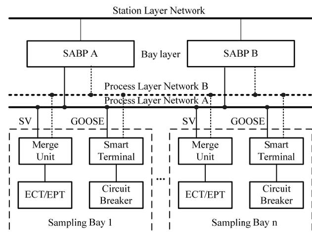
Fig.1. Schematic diagram of the centralized type SABP
