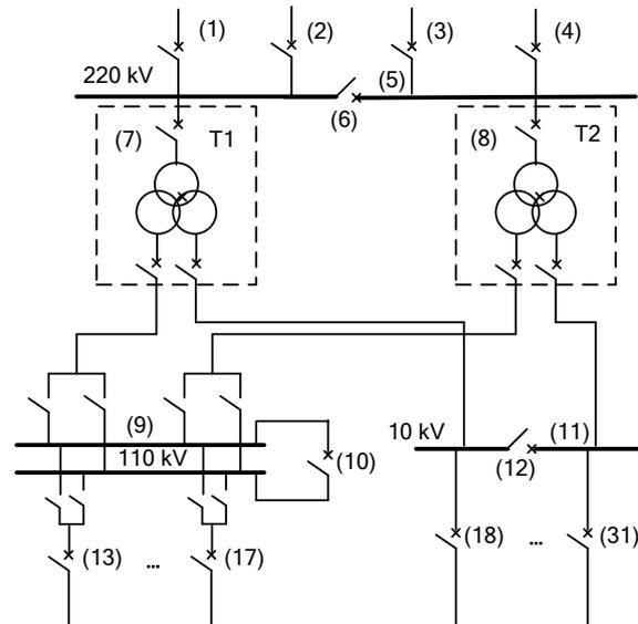
Fig.3. Main structure of a practical 220kV smart substation and its bay layout
