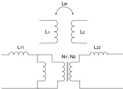
Fig.3. An Equivalent circuit of the contactless transformer
