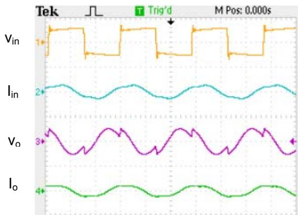
Fig.9. Experimental waveforms of the contactless system with 10 mm gap [ $V_{in} = 100$  V/div  $I_{in} = 5$ A/div  $V_o = 50$ V/div  $I_o = 5$ A/div]
