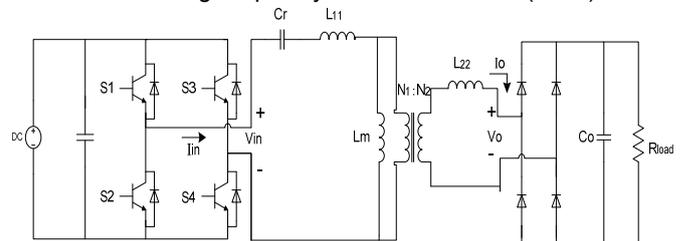
Fig.1. Series resonant converter
