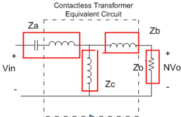
Fig.6. Equivalent circuit of the contactless transformer
