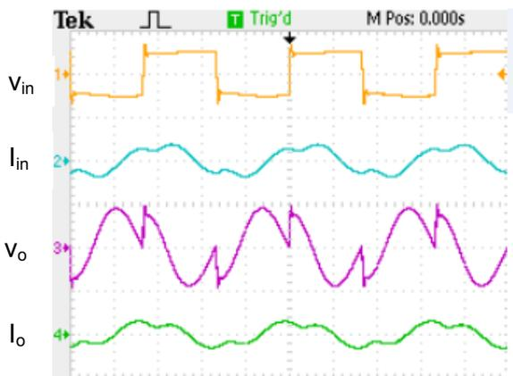
Fig.8. Experimental waveforms of the contactless system with 8mm gap [ $V_{in} = 100$  V/div  $I_{in} = 10$  A/div  $V_o = 50$  V/div  $I_o = 10$  A/div]
