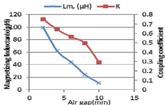
Fig.5. Contactless transformer parameters according to the air gap variation
