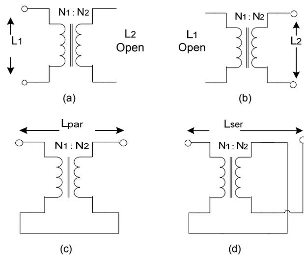
Fig.4. Measurement of transformer parameters, (a) primary side self-inductance, (b) secondary side self-inductance, (c) parallel inductance, (d) series inductance.
