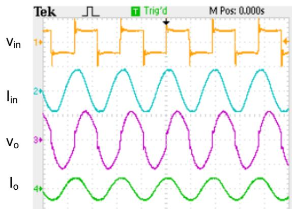
Fig.7. Experimental waveforms of the contactless system with 4mm gap [ $V_{in} = 100$  V/div  $I_{in} = 10$  A/div  $V_o = 50$  V/div  $I_o = 10$  A/div]
