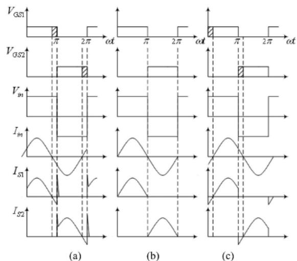
Fig.2. Resonant frequency characteristic waveforms with respect to switching and resonant frequency for (a)  $f_s < f_r$  (b)  $f_s = f_r$  (c)  $f_s > f_r$  [7]
