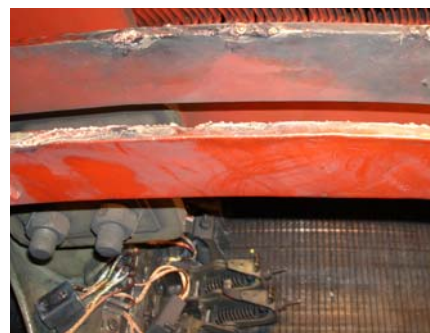
Fig.3. Destroyed bridge of brush-holder and commutator burnings
