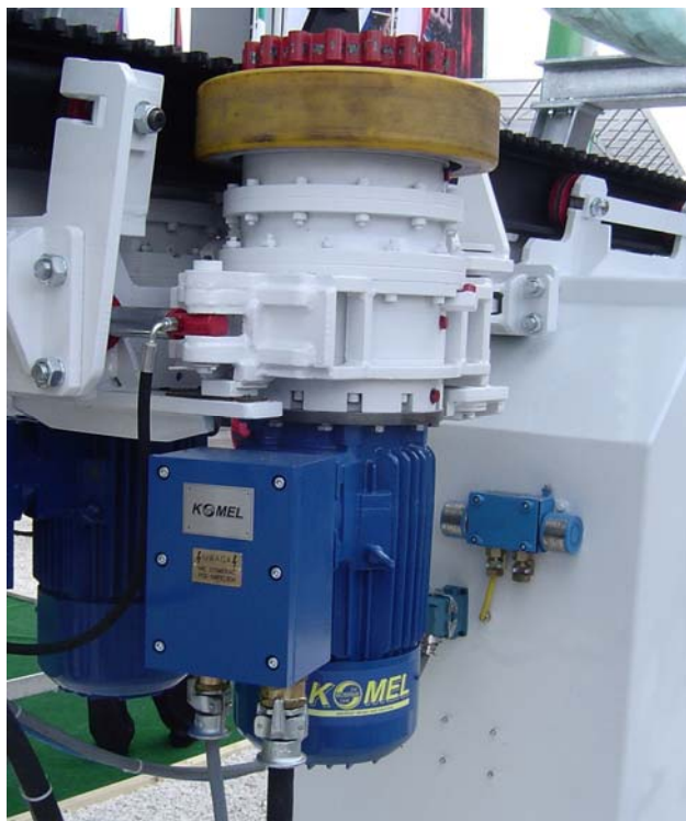
Fig.4. Electric mining motor SMwsPA132M6 type manufactured in BOBRME "Komel" , mounted in the GAD-1 drive
