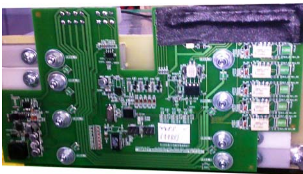
Fig. 6. Battery Management System (BMS) used in GAD-1 suspended drivetrain
