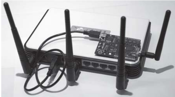
Fig. 8. The prototype of integrated router based on TP-Link 1043ND router and Zigduino board
