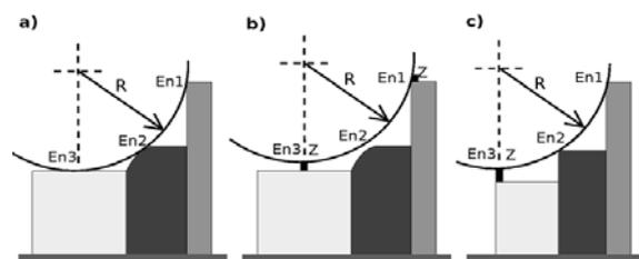
Fig. 1 Illustration of local conditions affecting the interception of lightning discharges by RSM
