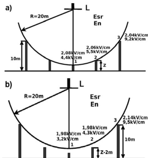
Fig.6 Examples of computing systems with structures: a) being in contact with sphere, b) lower in points 1, 2; En – electric field vector values (black) and the Esr - average electric field value (blue)
