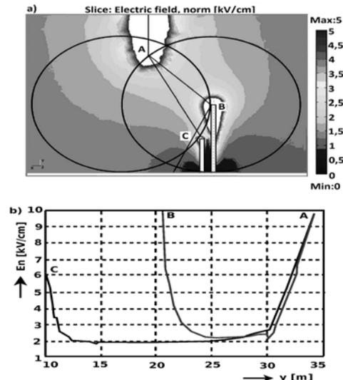
Fig.3 Field distribution: a) colored chart, b) field distribution between points A-B and A-C
