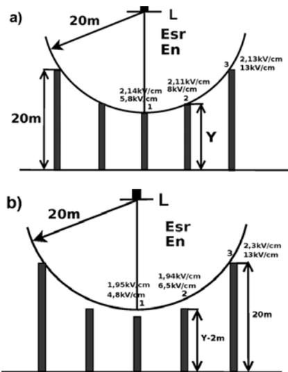
Fig.5 Examples of computing systems with structures: a) being in contact with sphere, b) lower in points 1, 2; En – electric field vector values (black) and the Esr - average electric field value (blue)
