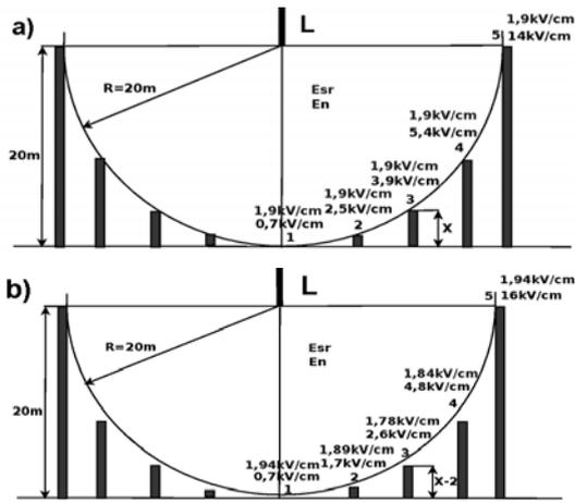
Fig.4 Examples of computing systems with structures: a) being in contact with sphere, b) lower in points 2, 3, 4; En – electric field vector values (black) and the Esr - average electric field value (blue)
