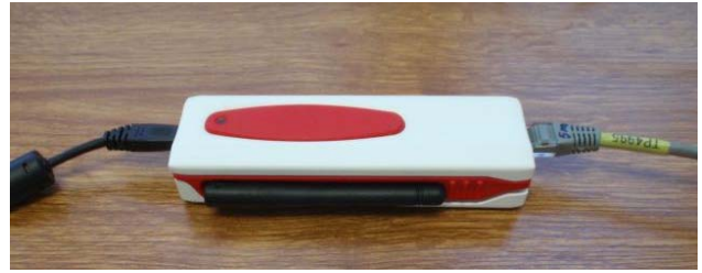
Fig. 9. Housing Gumstix computer Verdex developed custom solutions for the needs of the project – reality
