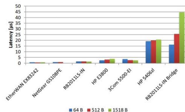
Fig. 7. Measured switching latencies for Ethernet 1000Base-T.
