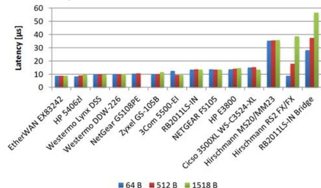
Fig. 5. Measured switching latencies for Ethernet 10Base-T.
