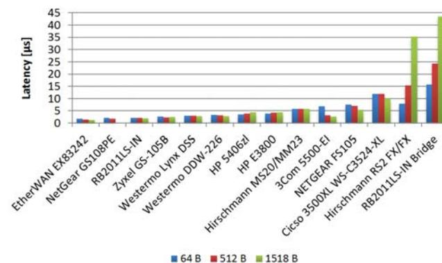
Fig. 6. Measured switching latencies for Ethernet 100Base-TX.
