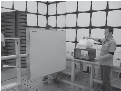
Fig. 1. Antenna and near field sensor in the testing site
