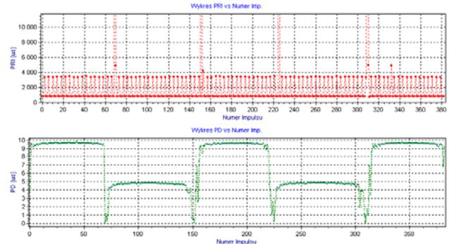
Fig.15. Changing PD values after each antenna scan – airborne surveillance radar
