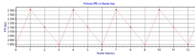
Fig.9. PRI stagger regular (3-element, 3-position) – land-based search radar
