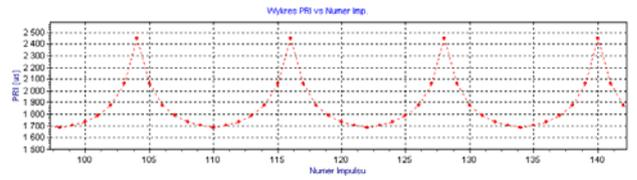
Fig.6. PRI sliding non-linear – land-based altimeter
