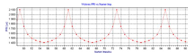
Fig.11. PRI stagger complex (7-element, 12-position) – air and surface search radar
