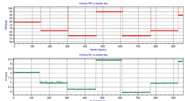
Fig.16. Synchronous changes values of PRI and PD – airborne warning radar
