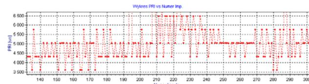
Fig.13. PRI discrete jitter – airborne search radar
