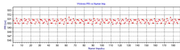
Fig.12. PRI continuous jitter – naval surface search radar
