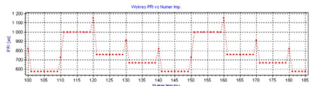
Fig.8. PRI dwell and switch (4-dwell, non-zero time to switch) – naval surface search radar
