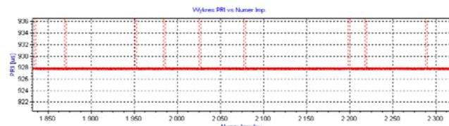
Fig.2. PRI stable – naval surface search radar
