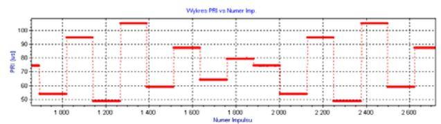
Fig.7. PRI dwell and switch (9-dwell, zero time to switch) – multi-function fighter-plane radar
