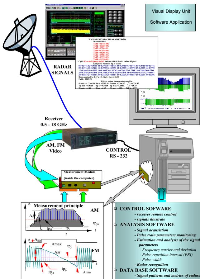
Fig.1. A structure of electronic recognition system
