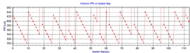
Fig.5. PRI sliding linear – naval search radar
