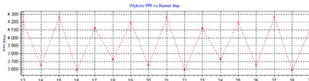
Fig.10. PRI stagger irregular (6-element, 6-position) – land-based search radar
