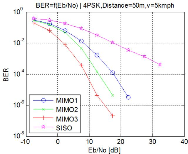
Fig. 5. MIMO in comparison to SISO for 4PSK (simulation in Matlab)
