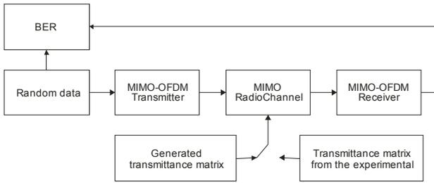
Fig.4. Block diagram of the MIMO link Matlab simulation model
