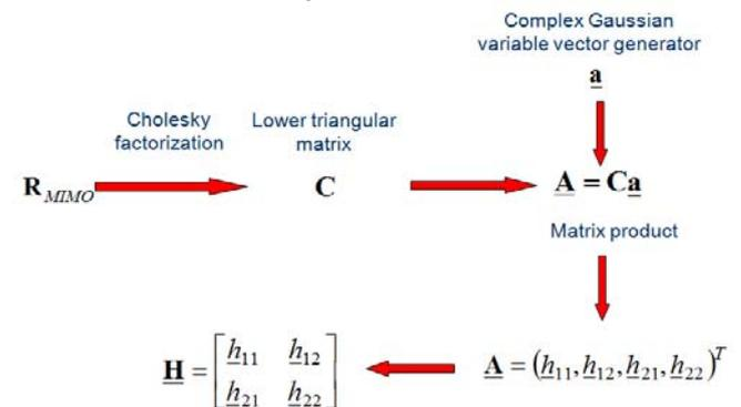
Fig.3. MIMO channel simulation algorithm [10]
