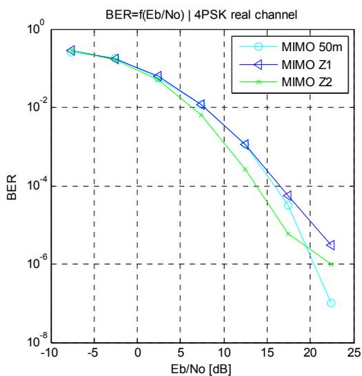
Fig.8. MIMO channel with real parameters of transmittance matrix for 3 different user locations (50m – LOS; Z1, Z2 – NLOS)
