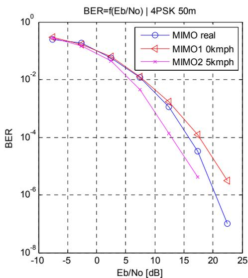
Fig.9. Comparison of MIMO channel simulation results (for user speed: MIMO1 v=0kmph, MIMO2 v=5kmph) with real environment (MIMO real, v≈2+3kmph)
