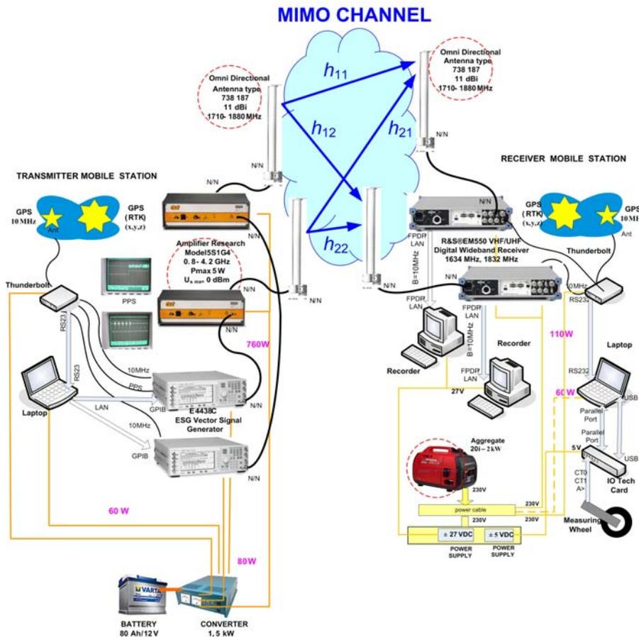
Fig.7. Structure of the test-bed for quality assessment of MIMO system
