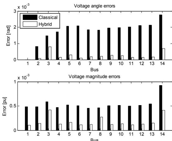
Fig. 2. Voltage angle and magnitude errors for the IEEE 14 - average values of 100 Monte Carlo simulations
