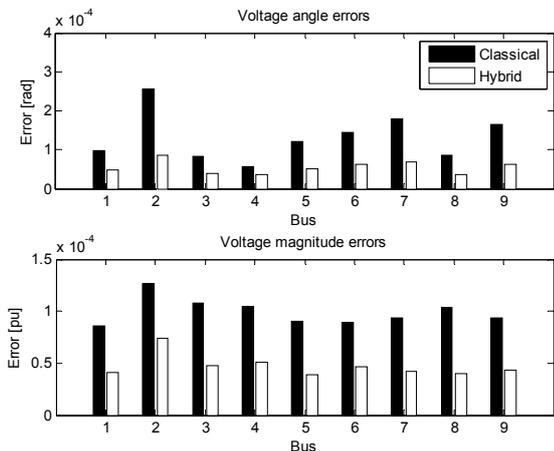
Fig. 5. Voltage angle and magnitude errors for the Croatian TPS - average values of 100 Monte Carlo simulations
