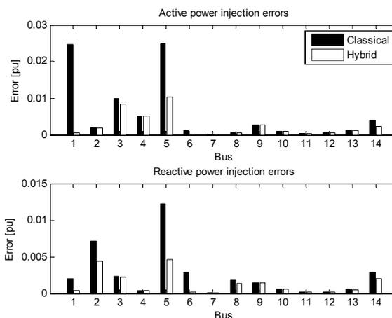
Fig. 3. Power injection errors for the IEEE 14 - average values of 100 Monte Carlo simulations
