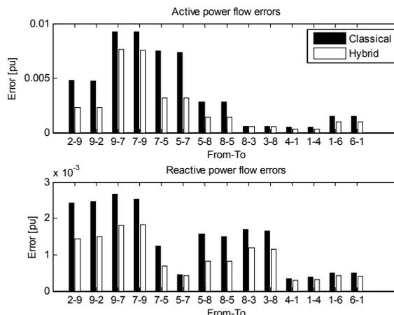
Fig. 7. Power flow errors for the Croatian TPS - average values of 100 Monte Carlo simulations
