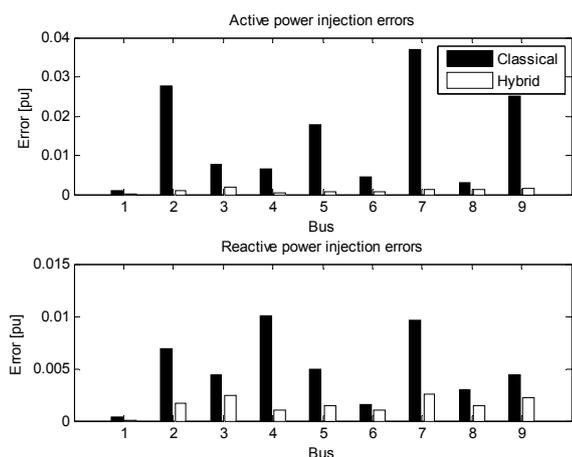
Fig. 6. Power injection errors for the Croatian TPS - average values of 100 Monte Carlo simulations
