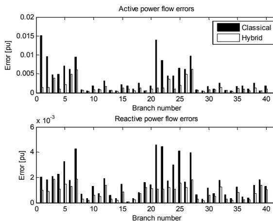
Fig. 4. Power flow errors for the IEEE 14 - average values of 100 Monte Carlo simulations
