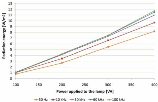
Fig. 3. Characteristics of radiation energy variation depending on power applied to the lamp for various values of frequency
