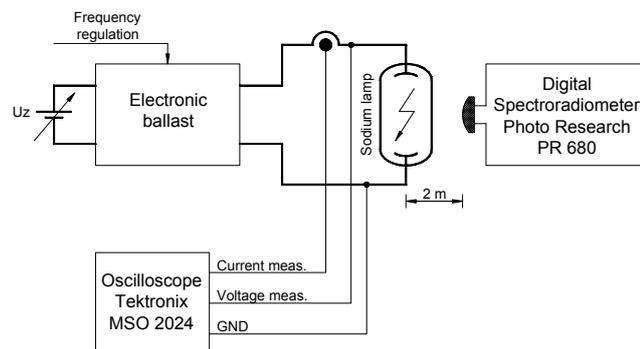
Fig. 1. Diagram of the test station for spectrum and light radiation energy
