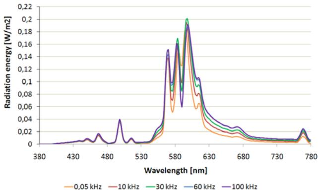
Fig. 9. Spectral characteristics of sodium lamp for  $S=400$  VA
