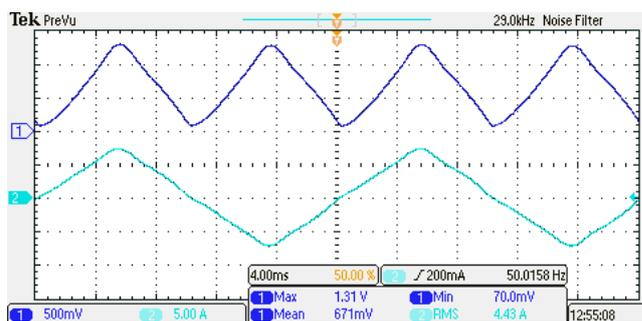
Fig. 14. Functions of luminous flux and supply current of sodium lamp for the power of  $S=400$  VA and  $f=50$  Hz. Channels: CH1-voltage from photo-detector, CH2- lamp supply current
