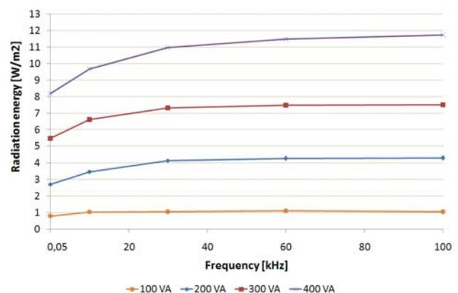
Fig. 2. Characteristics of radiation energy variation depending on frequency of power supply for various values of power applied to the sodium lamp.
