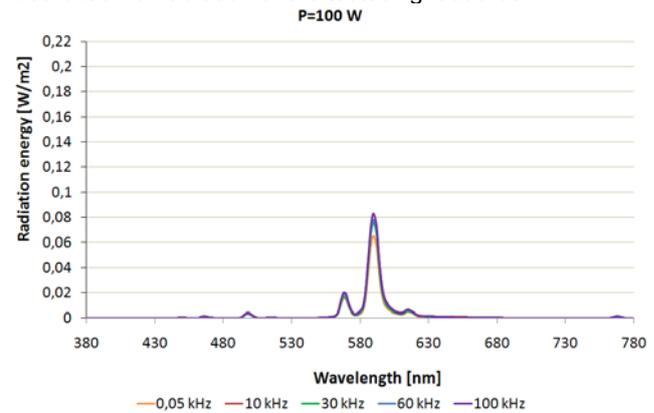
Fig. 6. Spectral characteristics of sodium lamp for  $S=100$  VA
