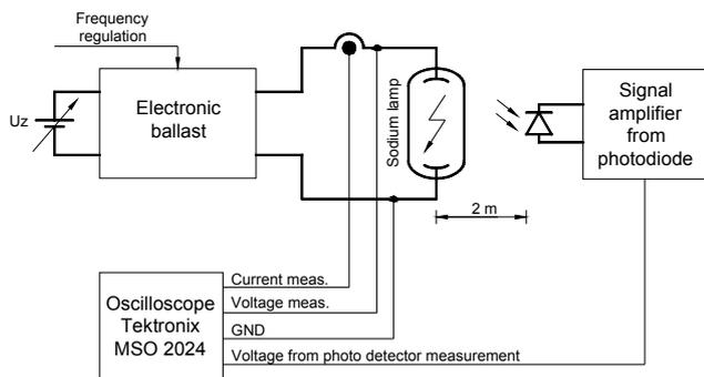
Fig. 10. Light pulsation test station diagram
