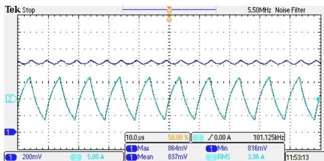
Fig. 11. Functions of luminous flux and supply current of metal halide lamp for the power of  $S=400$  VA and  $f=100$  kHz. Channels: CH1-voltage from photo-detector, CH2- lamp supply current
