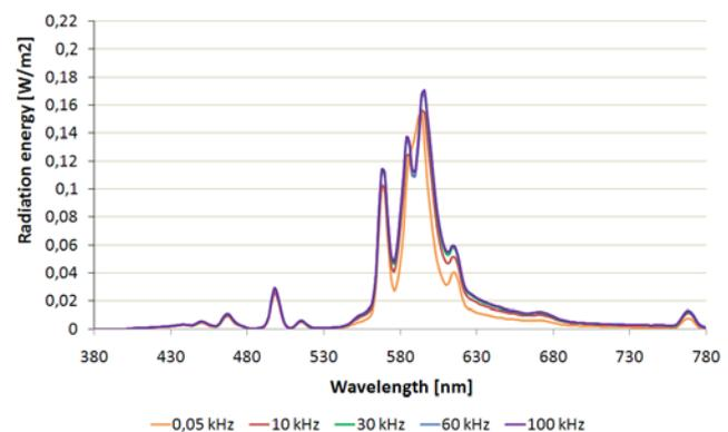
Fig. 8. Spectral characteristics of sodium lamp for  $S=300$  VA
