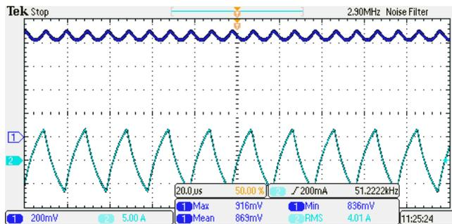
Fig. 12. Functions of luminous flux and supply current of metal halide lamp for the power of  $S=400$  VA and  $f=50$  kHz. Channels: CH1-voltage from photo-detector, CH2- lamp supply current
