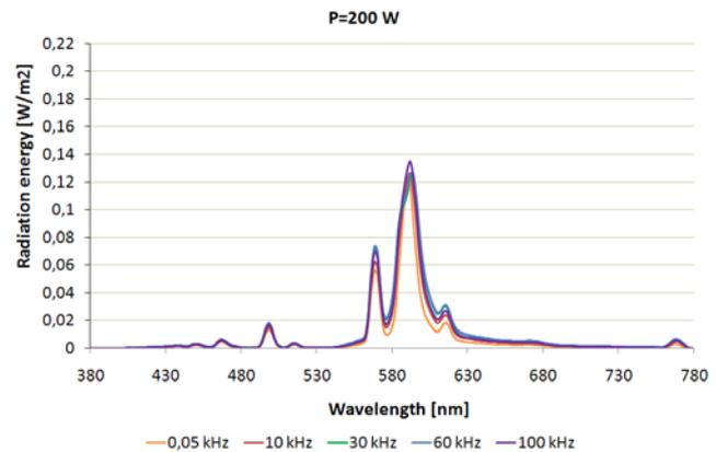
Fig. 7. Spectral characteristics of sodium lamp for  $S=200$  VA
