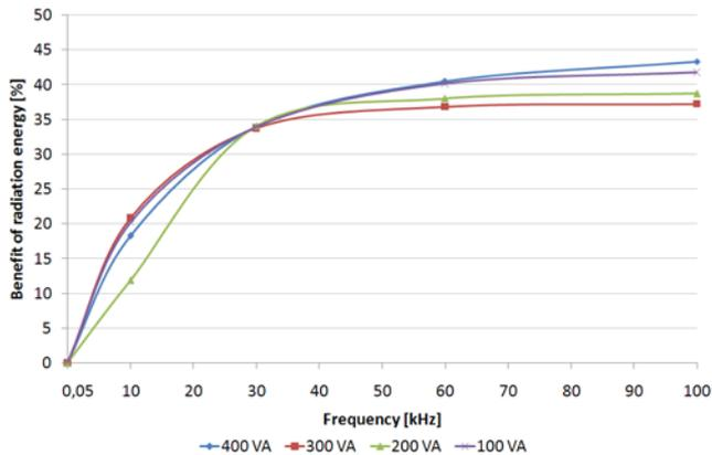
Fig. 4. Functions of benefit of radiation energy values depending on the power supply frequency of the lamp for various values of power applied to the lamp
