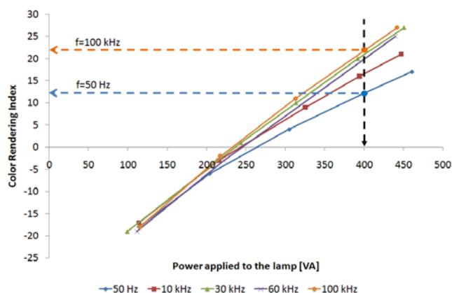
Fig. 16. Functions of CRI parameter value against power applied to the sodium lamp at various voltage frequencies of the lamp.
