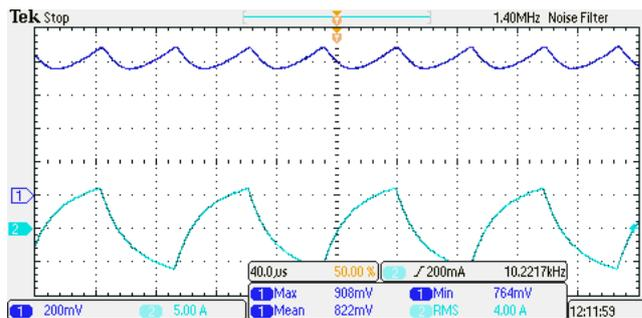
Fig. 13. Functions of luminous flux and supply current of metal halide lamp for the power of  $S=400$  VA and  $f=10$  kHz. Channels: CH1-voltage from photo-detector, CH2- lamp supply current
