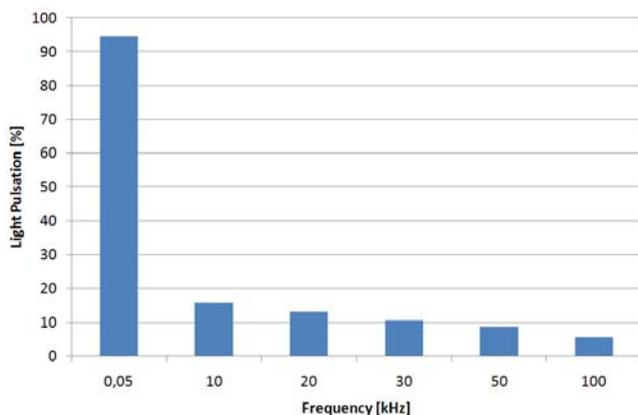
Fig. 15. Values of light pulsation when supplying sodium lamp with the power of  $S=400\text{VA}$  at various values of voltage frequency (graphic interpretation of table 1)
