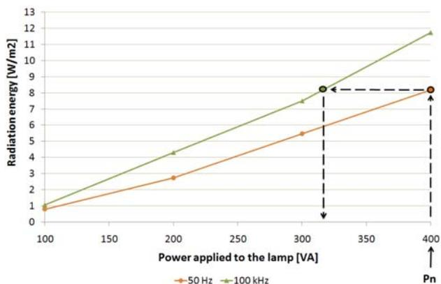
Fig. 5. Functions of radiation energy for frequencies  $f=50$  Hz and  $f=100$  kHz.
