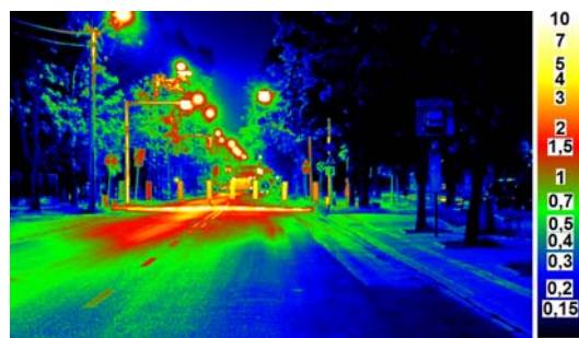
Fig. 13. Luminance measurement of objects from the first observation direction (logarithmic scale \log_2 , unit \text{cd/m}^2 ) in the case of pedestrian crossing lighting by means of light frames type 2
