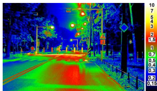
Fig. 14. Luminance measurement of objects from the second observation direction (logarithmic scale \log_2 , unit \text{cd/m}^2 ) in the case of pedestrian crossing lighting by means of light frames type 2
