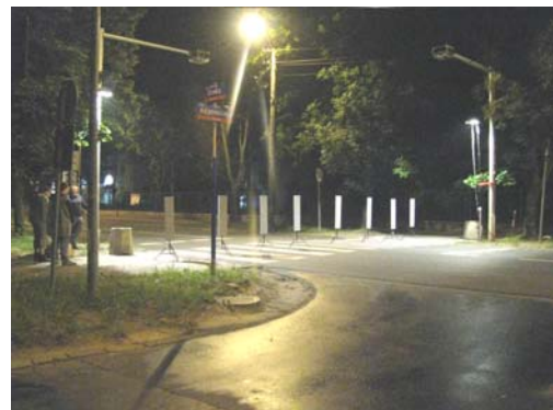
Fig. 7. Light frames type 1 temporarily installed on pedestrian crossing
