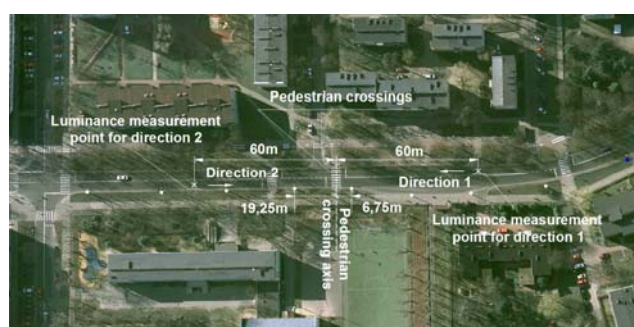
Fig. 1. Placement of street lighting with regard to pedestrian crossing with indicated directions of measurement [7]
