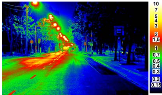
Fig. 3. Luminance measurement of objects from the first observation direction (logarithmic scale \log_2 , unit \text{cd}/\text{m}^2 )
