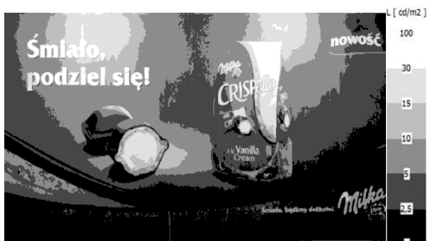
Fig. 10. An example of luminance distribution on the surface of a traditional billboard
