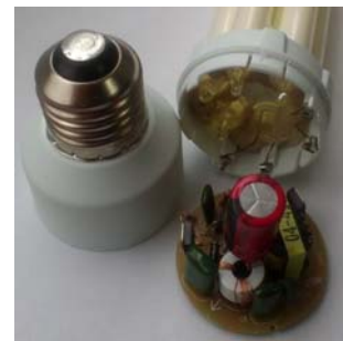
Fig. 3. Compact fluorescent lamp circuit exemplary practical implementation
