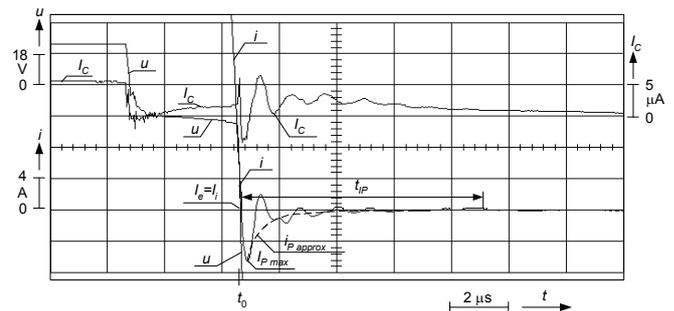
Fig. 4. The exemplary oscillogram of the arc current  $i$ , voltage on the contacts  $u$  and the collector current of the RFA  $I_C$  shortly before and after current zero (time instant  $t_0$ ),  $t_{Pmax}$  – the time of flowing the post-arc current; explanation of other symbols in the text
