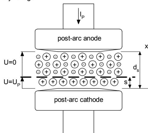
Fig. 2. Sketch diagram of the space charge distribution (ions and electrons) and growth of charge after current zero in vacuum;  $s$  – thickness of ion layer at post-arc cathode,  $d_s$  – the whole contact gap,  $U=0$  – recovery voltage on the neutral plasma,  $U=U_P$  – transient recovery voltage on the ion layer,  $x$ -marking of axis,  $I_P$  – total post-arc current, (explanation remaining symbols in the text)
