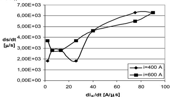
Fig. 8. The diagrams of estimated speed of the ion layer displacement  $ds/dt$ , versus rate of rise of the counter-current  $di_k/dt$
