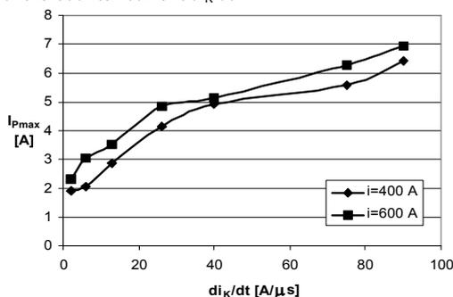
Fig. 6. The diagrams of the measured peak post-arc current  $I_{Pmax}$  versus rate of rise of the counter-current  $di_k/dt$
