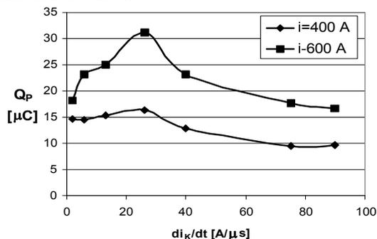
Fig. 5. The diagrams of calculated residual charge  $Q_P$  versus rate of rise of the counter-current  $di_k/dt$
