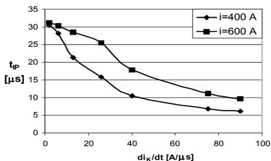
Fig. 7. The diagrams of the measured time  $t_{IP}$  of the flowing post-arc current  $I_P$  (Fig. 1 and Fig. 4) versus rate of rise of the counter-current  $di_k/dt$
