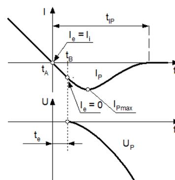
Fig. 1. Illustration of the current flow after zero the passage in vacuum [10];  $I_e$ ,  $I_i$  – electron and ion current respective;  $I_P$  – total post-arc current,  $t_{IP}$  – the time of post current flow,  $U_P$  – transient recovery voltage
