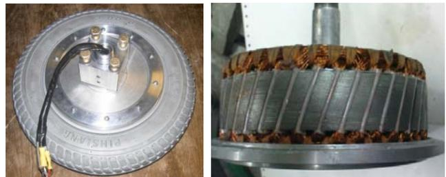
Fig. 1. Physical motor: a) in-wheel assembly, b) winding and skewed stator.
