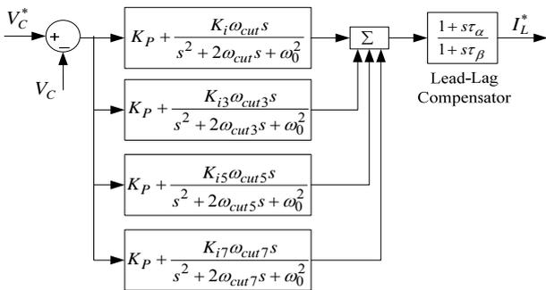
Fig. 8. Proportional-multiresonant controller for fundamental and harmonic (third, fifth and seventh) components
