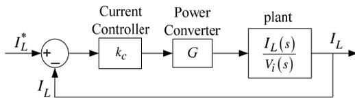
Fig. 4. Inner current loop and plant.
