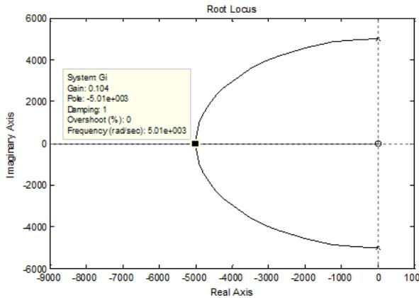
Fig. 5. Root locus plot of current loop.
