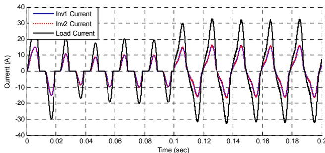
Fig. 14. One phase current waveform of each inverter with equal ratings and total drawn phase current.
