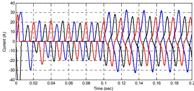
Fig. 13. The three-phase current of nonlinear and unbalanced loads at the output of parallel four-leg inverters.
