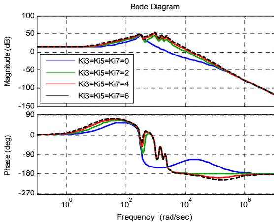
Fig. 9. Bode plot of voltage loop for different values of  $K_{i3}$ ,  $K_{i5}$  and  $K_{i7}$  (in Ohm inverse).
