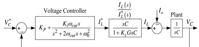
Fig. 7. Proportional-resonant controller for fundamental component.
