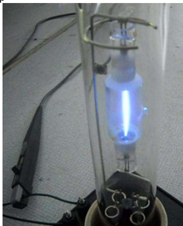
Fig. 8. View of the filament and of the high voltage pulse ionizing gas before ignition
