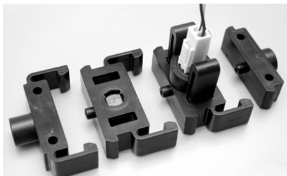
Fig. 3. Modular flow packages for ISFET and REFET sensors.
