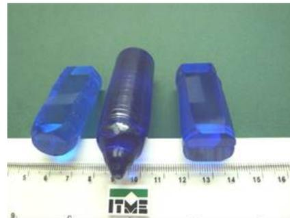
Fig. 1. An exemplary two Co-doped MALO boules prepared for testing : two pairs (end faces and on the perimeter, respectively) of surfaces have been polished for optical testing. In the center one can see "as grown" boule (just after pulling).
