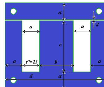
Fig.2. Geometrical cross-section of the core
