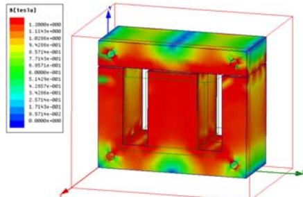
Fig.3. Magnetic flux density distribution,  $I_n = 1.15 A$
