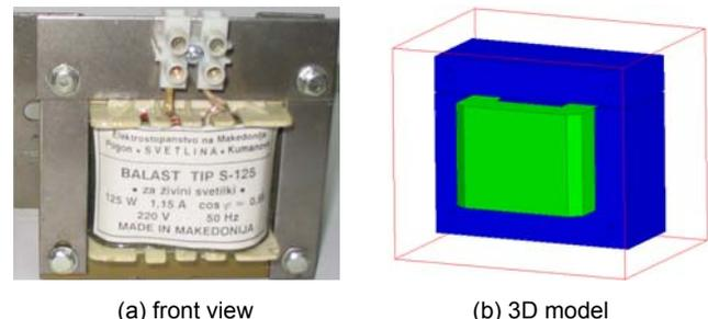
Fig.1. Generic model – original E-I core inductor
