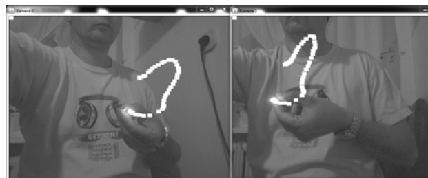
Fig.4. Output video frames of two synchronized Eye cameras with red LED marker tracing paths
