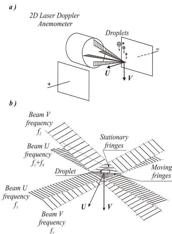
Fig.2. a) single droplet size and velocity (i.e. electrical mobility) PDA-based measurement arrangement, b) schematic of forming of interference patterns
