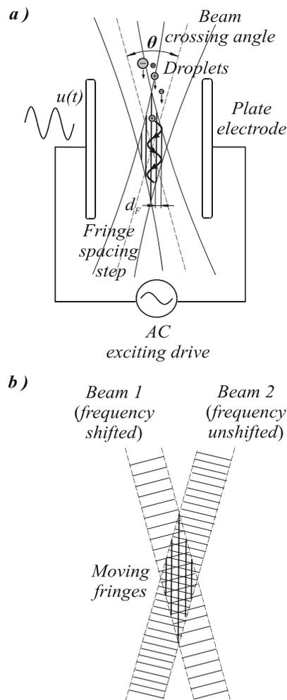
Fig.1. a) single droplet size and velocity (i.e. electrical mobility) LDV-based measurement arrangement, b) schematic of interference pattern forming
