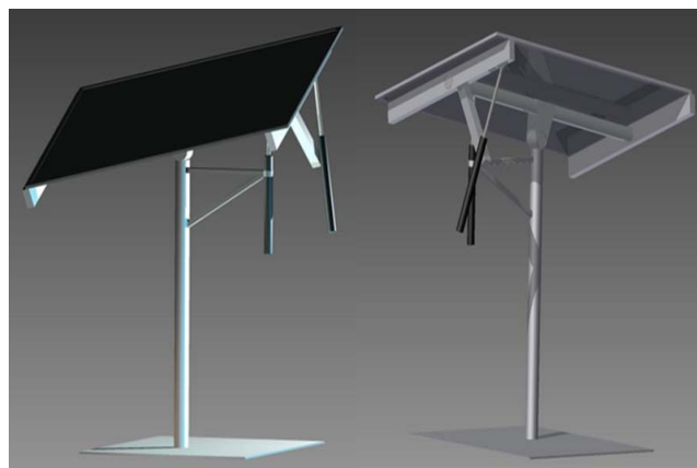
Fig.3. Design of two - axis tracking unit installed on the roof of the Faculty of Electrical Engineering Poznan University of Technology building
