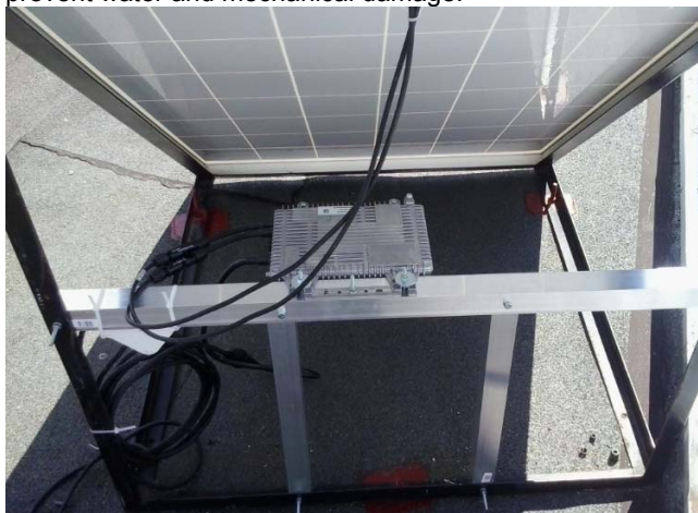
Fig.2. Stationary system with photovoltaic module, radiation power density sensor and microinverter
