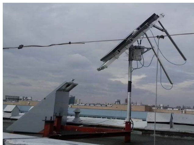
Fig.4. Two - axis tracking system with photovoltaic module, radiation power density meter and microinverter
