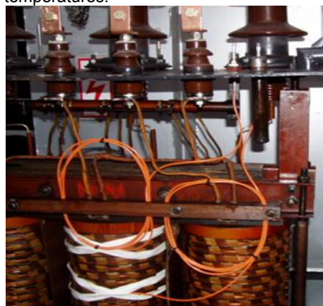
Fig.3. View of the optical detectors positioning (covered by white stripes)
