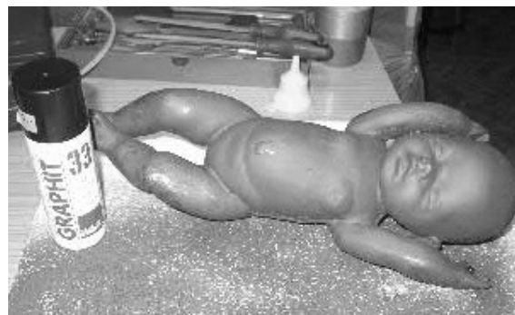
Fig.5. Thermal manikin covered with graphite (high emissivity) spray coating
