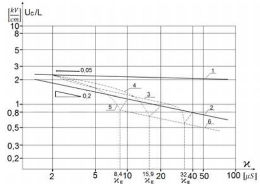
Figure 7. Pollution characteristics of a composite insulator.
