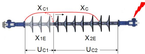
Fig. 6 Ignition (in section  $X_{1E}$ ) and propagation of electric arc (in section  $X_{2E}$ ) correspond to the occurrence of a sudden flashover on a long rod composite insulator surface with non-uniformly distributed wettability. Critical voltages  $U_{C1}$  and  $U_{C2}$  have similar values and  $X_{C1}$ ,  $X_C$  are arcs that burn on  $X_{C1}$  section and on the whole insulator respectively.
