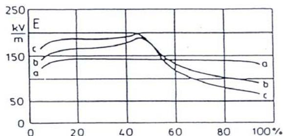
Fig. 2. Calculated distributions of the tangential component  $E_t$  of the electric field along the cylindrical insulator polluted with non-uniform layer. a) uniform layer on the entire surface of the insulator, b) non-uniform layer, conductivity relationship for layers on both halves of the insulator surface equals 1:2, c) Non-uniform layer, conductivity relationship for layers on both halves of the insulator surface equals 1:4
