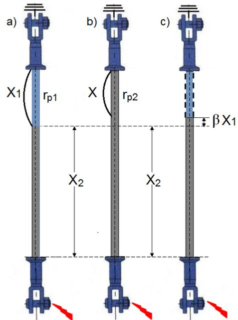
Fig. 5. The model cylindrical insulators of diversified values of surface pollution resistances per unit length  $r_{p1}$  and  $r_{p2}$ . a) insulator with a partial arc of  $X_1$  length b) insulator with a partial arc of  $X$  length c) equivalent insulator of a uniform pollution resistance per unit length  $r_{p2}$ .
