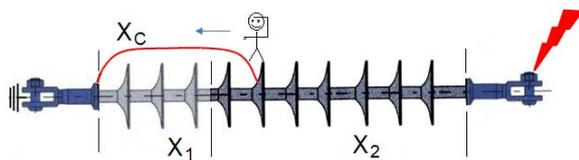
Fig. 4. Composite insulator of diversified wettability of sections of a creepage distance  $X_1$  and  $X_2$ , which correspond to surface conductivities  $\kappa_{p1}$  and  $\kappa_{p2}$  or resistances per unit length  $r_{p1}$  and  $r_{p2}$ . It has been assumed that  $X_C > X_1$ .
