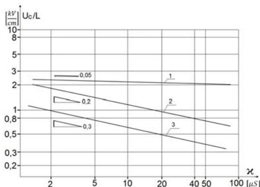
Fig. 1. Double-logarithmic scale pollution characteristics of long rod composite insulator (1, 2) and long rod porcelain insulator (3). 1. Characteristic for composite insulator with hydrophobic surface, 2. Characteristic for composite insulator with hydrophilic surface
