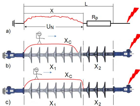
Figure 3. Electric model of a polluted insulator and a composite insulator of diversified wettability of surfaces of creepage distance sections ( $X_1$  and  $X_2$ ) and of surface conductivities  $\kappa_{p1}$  and  $\kappa_{p2}$  respectively:
