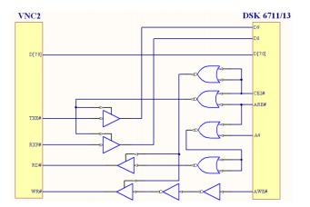
Fig. 1. The logic of the connection of the VNC2 to the DSK 6711/13 module
