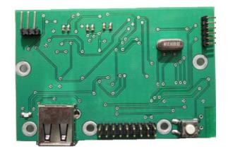
Fig. 2. The top layer of the designed USB module
