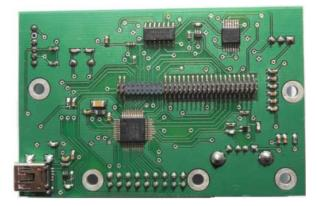
Fig. 3. The bottom layer of the designed USB module
