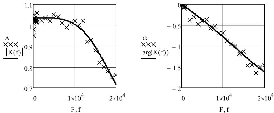
Fig. 4 Determined frequency characteristics in MathCad program.
