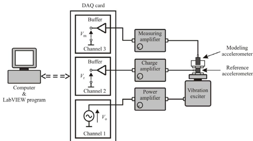
Fig. 1. Measuring system for frequency characteristics determination.
