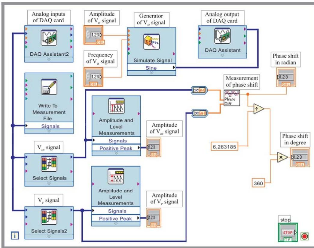
Fig. 3. Diagram of measuring system intended for determination of both frequency characteristics.
