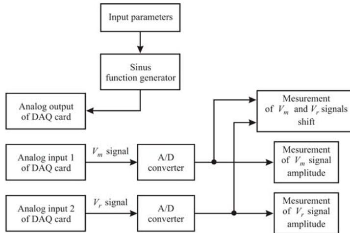
Fig. 2. Diagram of measuring system intended for determination of both frequency characteristics
