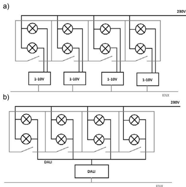
Fig. 2. Outline of the connection of dimmers for light fixtures in the standard: a) 1-10V, b) DALI
