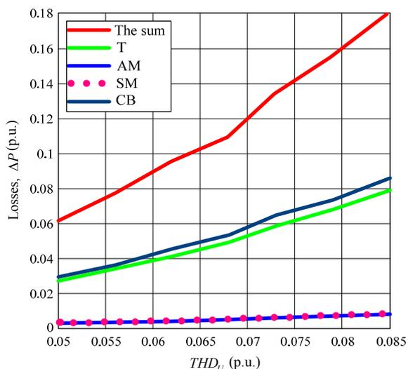
Fig. 5. The diagram of dependences of relative additional power losses in network's components upon  $THD_U$ , if three phase-three phase 6-pulse cycloconverter is the source of distortion
