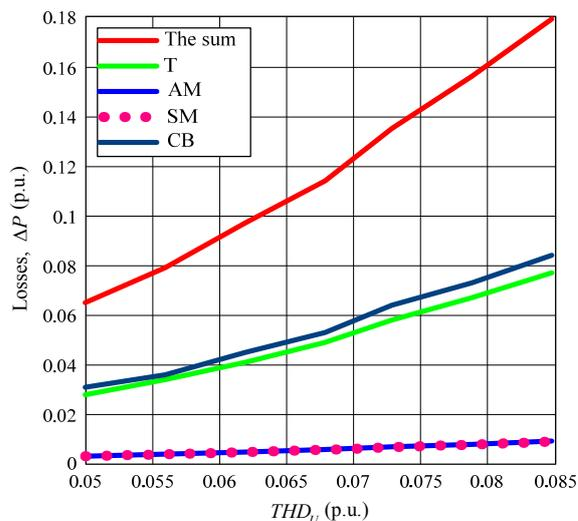
Fig. 4. The diagram of dependences of relative additional power losses in network's components upon  $THD_U$ , when a 6-pulse converter is the source of distortion
