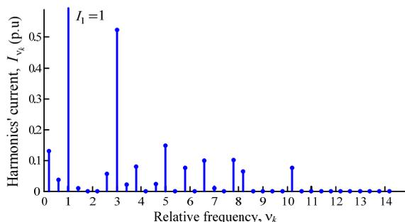
Fig. 3. Amplitude spectrum of the input current of three phase bridge 6-pulse cycloconverter with sinusoidal control law;  $f_{out} = 20$  Hz
