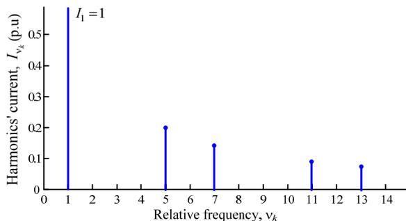
Fig. 2. Amplitude spectrum of the input current of 6-pulse frequency converter
