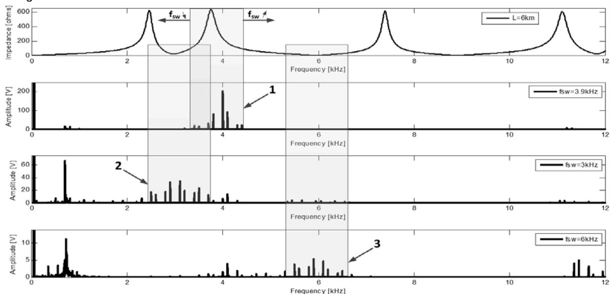
Fig.2. Network impedance for 6 km cable length and harmonics spectrums for three cases: (1) - rated  $f_{sw}$ , (2) - lower  $f_{sw}$ , (3) - higher  $f_{sw}$
