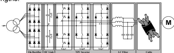
Fig.1. Three-level NPC inverter feeding the induction motor drive via the cable connection
