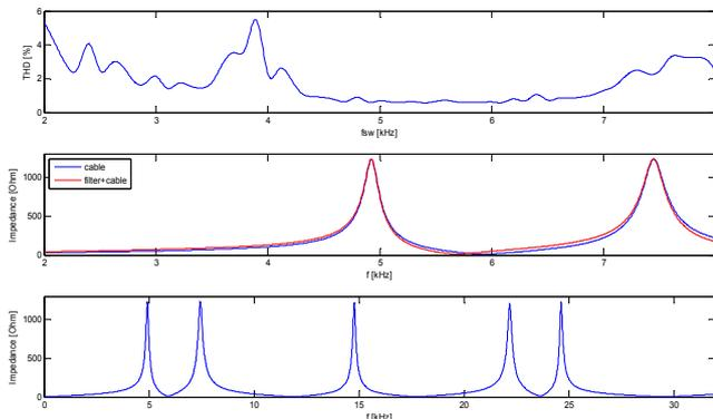
Fig.3. THD dependence on switching frequency and impedance curves for various cable lengths  $l = 3$  km,
