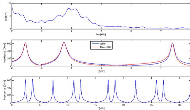
Fig.4. THD dependence on switching frequency and impedance curves for various cable lengths  $l = 6$  km,
