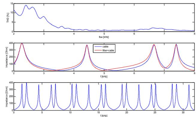
Fig.5. THD dependence on switching frequency and impedance curves for various cable lengths  $l = 10$  km
