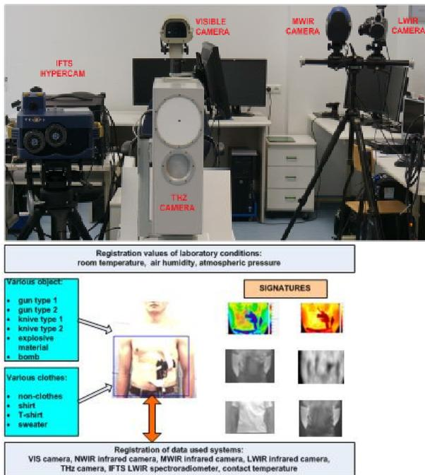
Fig.1. The systems used during the measurements and methodology of signature registration
