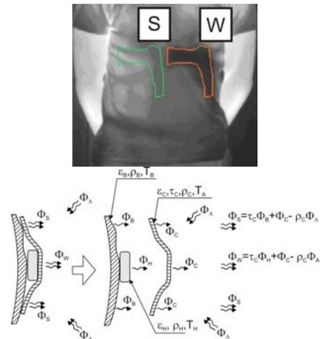
Fig.3. Thermal image of clothing surface with and without an object underneath, thermal radiation model in hidden object detection
