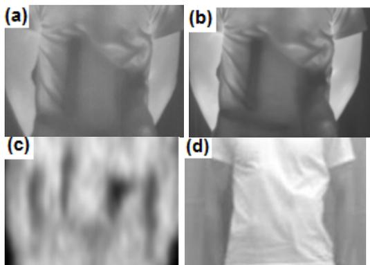
Fig.2. Complementary images; (a) LWIR image, (b) MWIR image, (c) THz image, (d) VIS image with hidden gun and a metallic tube
