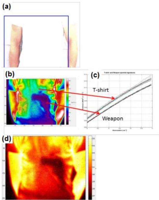
Fig.6. Analysis of sample data registered by IFTS HyperCam T-shirt: visible (a), spectral image (b), spectral radiance (c), broadband image calculate from spectral datacubes (d)
