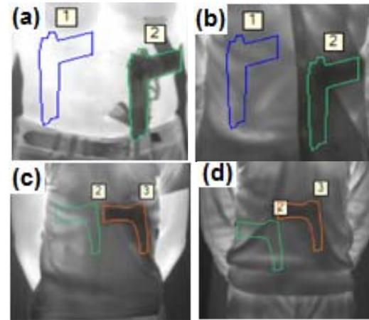
Fig. 5. Analysis of sample data registered by MWIR camera, (a) naked body, (b) shirt, (c) T-shirt, (d) sweater. Gun type1 on images (a) and (b), gun type 2 on images (c) and (d)
