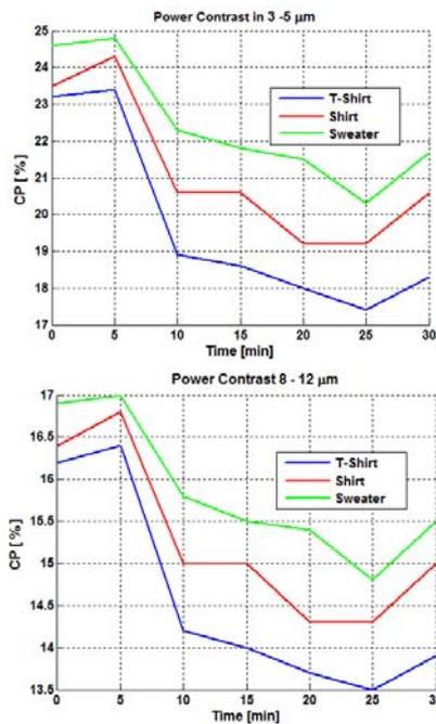
Fig.4. Calculation of power contrast for T-shirt, shirt, sweater in 3-5 μm and 8-12 μm region
