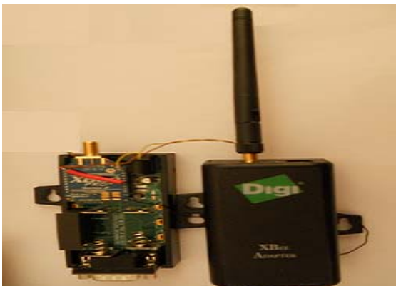
Fig. 6. Photograph of the XBee PRO ZB RS-232 Adapter (inside and outside) with external antenna
