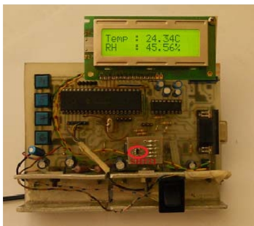
Fig. 2. Photograph of the PCB with SHT21 sensor
