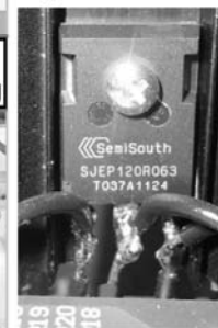
Fig. 7. The laboratory setup with proposed 50 kHz SiC-based DHB converter with 2 kW power planar transformer: circuit schematic (a); the overall view (b); investigated SiC MOSFET (c) and SiC JFET (d).
