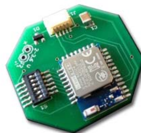
Fig 1. iBeacon with Bluetooth low energy module
