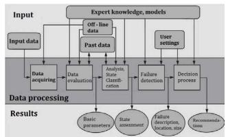
Fig. 1. The logical structure of the transformer state monitoring system [7].
