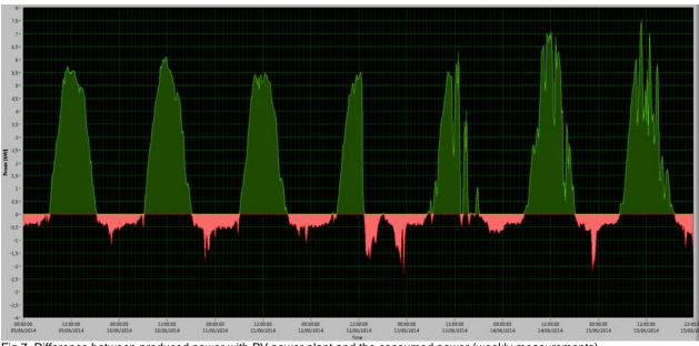
Fig.7. Difference between produced power with PV power plant and the consumed power (weekly measurements)
