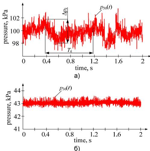
Fig. 6. Pressure variation curves  $p_{50}(t)$ ,  $p_{36}(t)$  at the pump output in the presence (a) and in the absence (b) of cavitation processes in the pipeline
