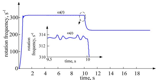
Fig. 4. Curves of variation of rotation frequency of the pump ED
