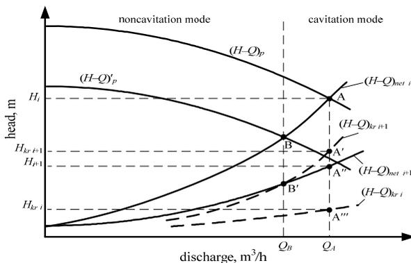
Fig. 1. Head-discharge characteristics of the pump and the pipeline
