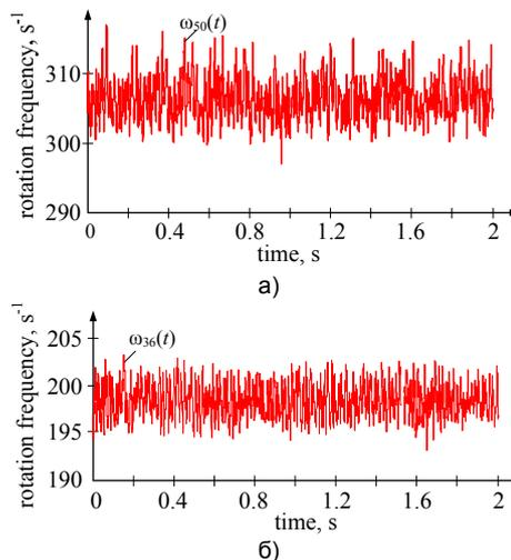
Fig. 7. Rotation frequency variation curves  $\omega_{50}(t)$ ,  $\omega_{36}(t)$  of the pump ED in the presence (a) and in the absence (b) of cavitation processes in the pipeline
