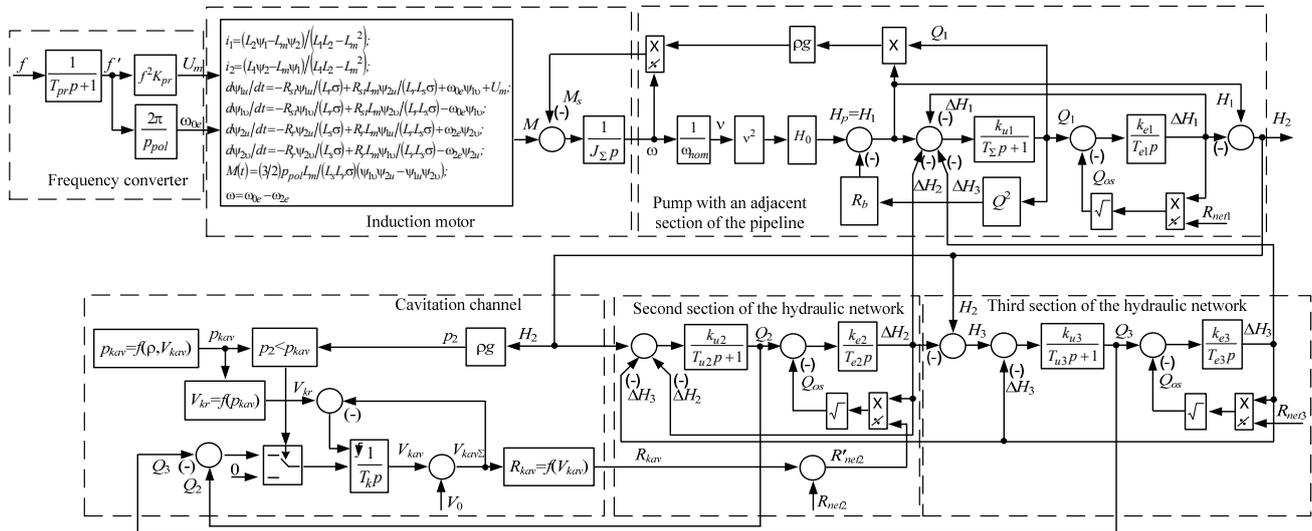
Fig. 2. Block diagram of a model of EHC with a cavitation channel
