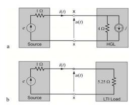
Fig. 2. Circuits with resistive HGL and LTI loads.
