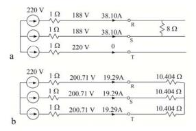
Figure 4. Circuits with balanced and unbalanced load.
