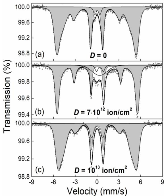
Fig.1. Mössbauer spectra of  $(\text{FeCoZr})_{58}(\text{CaF}_2)_{42}$  films – initial (a) as well as irradiated with fluences  $D = 7 \cdot 10^{12}$   $\text{ion/cm}^2$  (b) and  $D = 1 \cdot 10^{13}$   $\text{ion/cm}^2$  (c)
