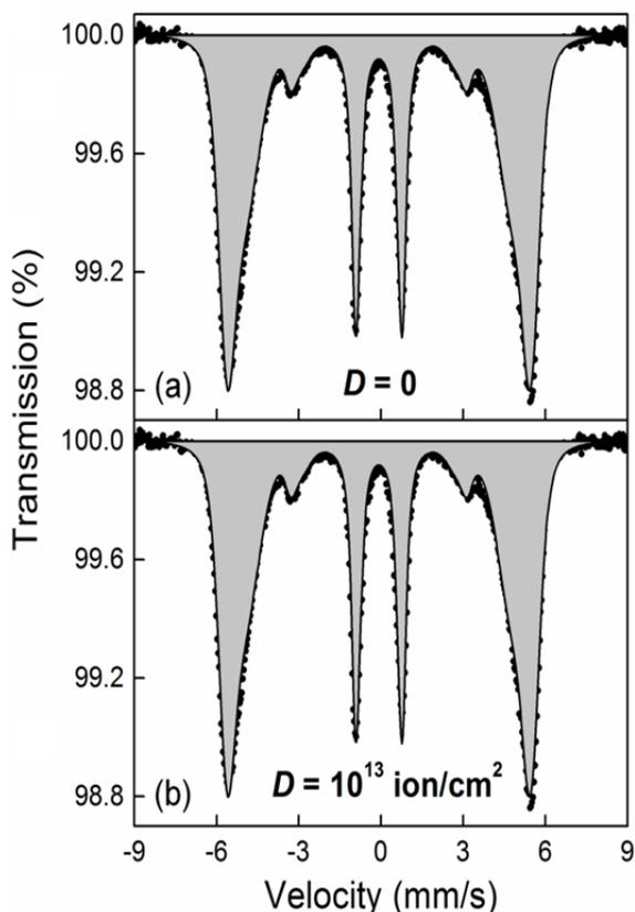
Fig.2. Mössbauer spectra of  $(\text{FeCoZr})_{73}(\text{CaF}_2)_{27}$  films – initial (a) and irradiated with fluence  $D = 1 \cdot 10^{13}$   $\text{ion/cm}^2$  (b)
