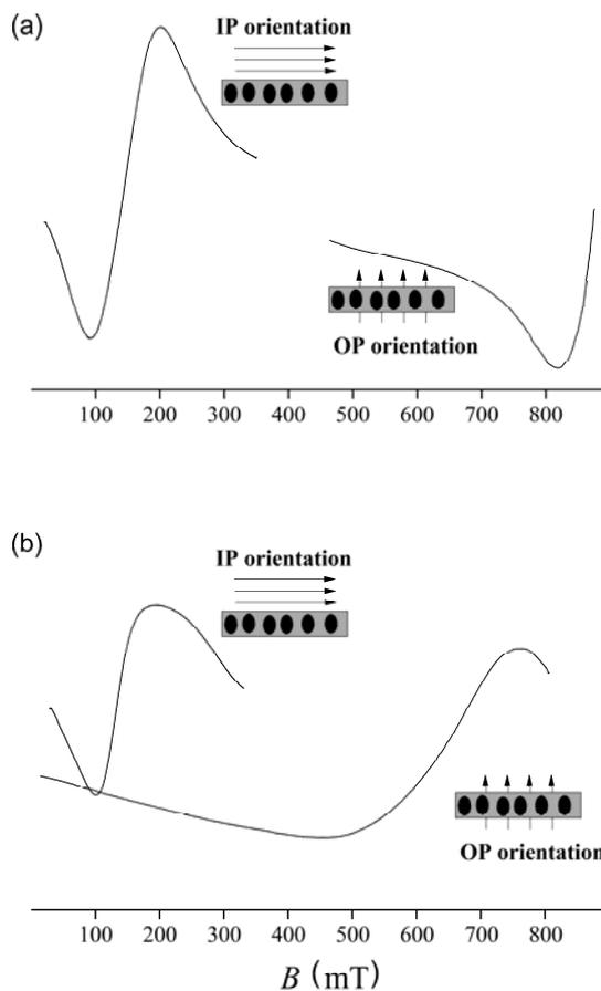
Fig.3. Magnetic resonance spectra of initial (a) and irradiated with  $D = 10^{13}$   $\text{ion/cm}^2$  (b)  $(\text{FeCoZr})_{58}(\text{CaF}_2)_{42}$  films measured at different orientations of external magnetic field
