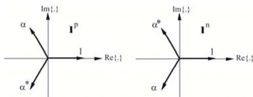
Fig. 3. Three-phase symmetrical unit vectors  $\mathbf{1}^p$  and  $\mathbf{1}^n$ .
