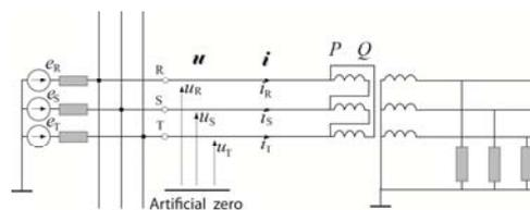
Fig. 1. Static load supplied from a three-wire line
