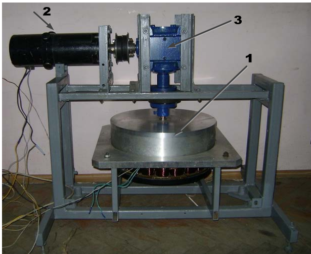
Fig. 4. Experimental stand for investigations of ETMEH: 1 – model of ETMEH, 2 – drive DC motor, 3 – reduction gear
