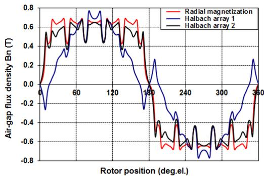
Fig. 6. Comparative characteristics of the normal component distribution for the air-gap magnetic flux density at no-load
