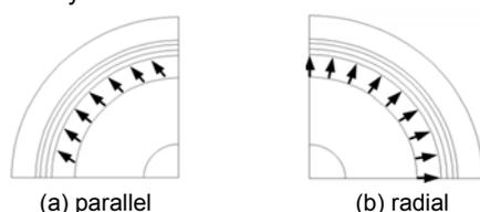
Fig. 1. Conventional magnetization of permanent magnets
