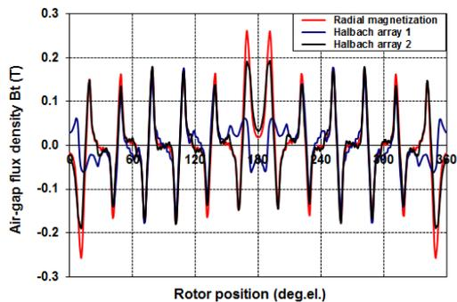
Fig. 7. Comparative characteristics of the tangential component distribution for the air-gap magnetic flux density at no-load
