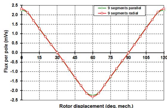
Fig. 4 Flux characteristics for conventional magnetization at no-load
