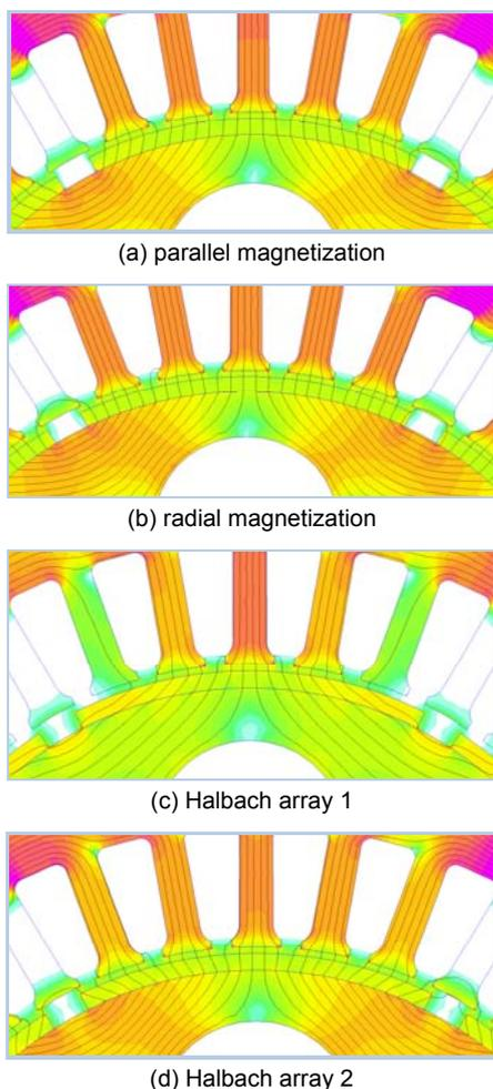
Fig. 3. Magnetic field at no-load for various types of magnetization
