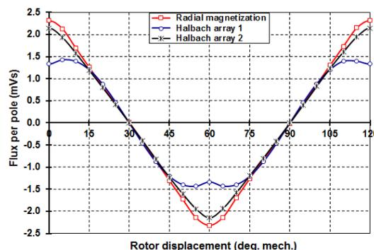
Fig. 5. Comparative characteristics of the magnetic flux per pole  $\Phi_p=f(\theta)$  at no-load
