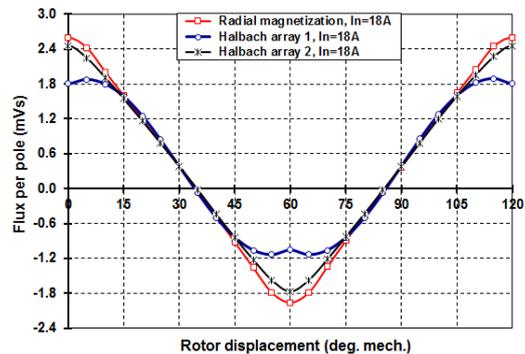
Fig. 8. Flux characteristics  $\Phi_p=f(\theta)$  at rated load  $I_n=18 A$
